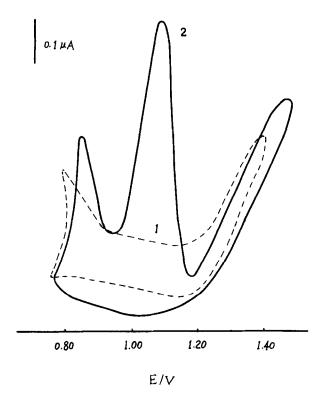
Fig. 6. Cyclic voltammograms of nitrite  $(NO_2^-)$ . The solution and other conditions are the same as those in Fig. 1.
