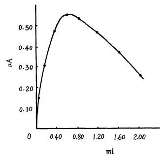
Fig. 2. Dependence of the anodic stripping peak current of nitrite ( $NO_2^-$ ) on the amount of 0.01 mol litre<sup>-1</sup> CTMAB. The solution and other conditions are the same as those in Fig. 1.
