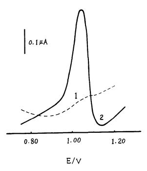
Fig. 1. Linear-sweep anodic stripping voltammograms of nitrite (NO<sub>2</sub><sup>-</sup>) after stirring for 90 s at +0.8 V. The solution contains  $1.2 \times 10^{-4}$  mol litre<sup>-1</sup> CTMAB and pH 3.9 BR buffer solution. Scan rate,  $100 \text{ mV s}^{-1}$ . Scan 1, no NO<sub>2</sub><sup>-</sup>; scan 2,  $0.20 \,\mu g \, m l^{-1} \, NO_2^{-}$  added.
