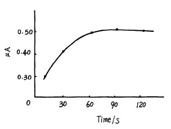
Fig. 5. Dependence of the anodic stripping peak current of nitrite  $(NO_2^-)$  on the accumulation time. The solution and other conditions are the same as those in Fig. 1.
