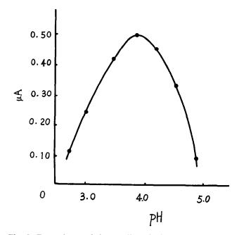
Fig. 3. Dependence of the anodic stripping peak current of nitrite  $(NO_2^-)$  on the pH value. The solution and other conditions are the same as those in Fig. 1.
