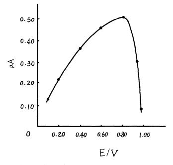
Fig. 4. Dependence of the anodic stripping peak current of nitrite  $(NO_2^-)$  on the accumulation potential. The solution and other conditions are the same as those in Fig. 1.
